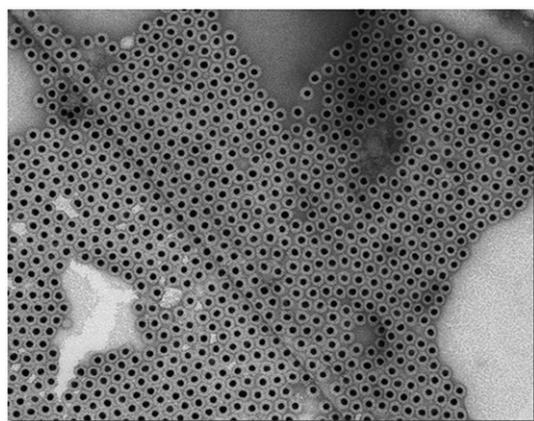
**Fig. 7** Transmission electron micrograph of virus-like particles (VLPs) containing gold nanoparticle cores (12 nm diameter) instead of RNA. VLPs can be efficiently assembled if the nanoparticles are pre-coated with a covalently bound carboxy-terminated PEG layer.
