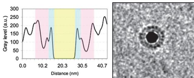
**Fig. 8** Cryo-TEM picture of a VLP containing a 12 nm, PEG-coated gold nanoparticle and cross-section through the center with different grey levels corresponding to different layers (gold, PEG, capsid protein) approximately marked in color. Note that despite the faceted character of the nanoparticle, the protein coat preserves a regular pattern of capsomeres and a quasi-spherical aspect.
